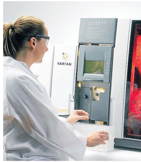
Varian's innovation in Atomic Absorption Spectroscopy allows rapid element analysis for environmental and industrial samples, particularly in the determination of toxic contaminants in foods and the environment. Varian Australia's Mulgrave operations achieve export sales of over $150 million a year with over 90% of production exported.
